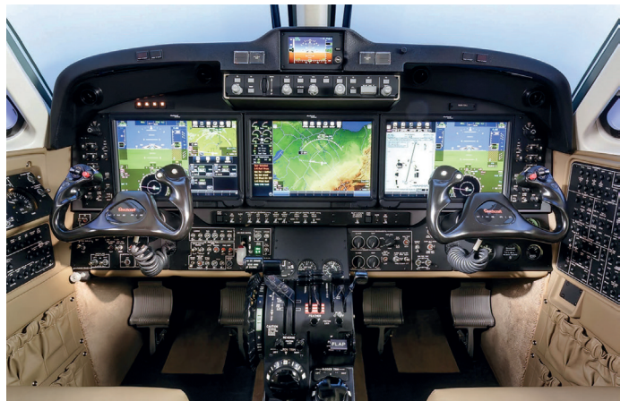
The King Air 360 is the latest version of Textron's Aviation pressurized twin-engine turboprop. It is fitted with the latest version of the Collins Proline Fusion suite and autothrottles.
