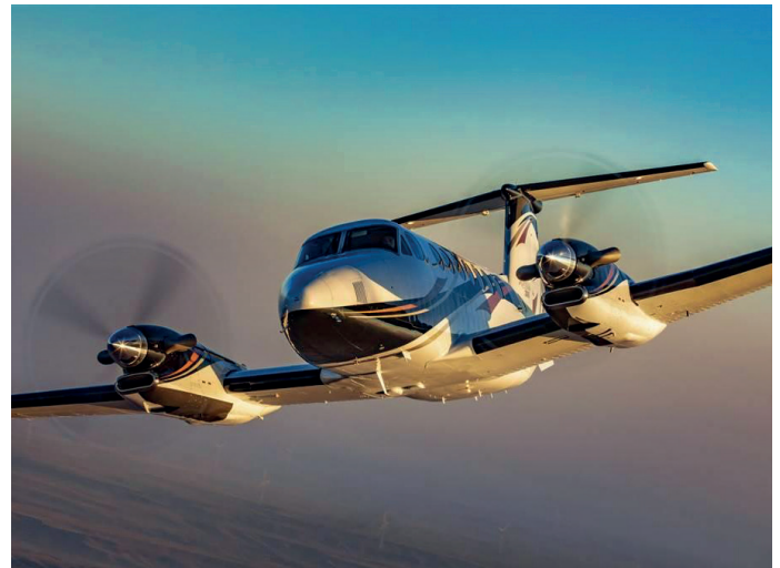
The King Air 360 is the latest version of Textron's Aviation pressurized twin-engine turboprop. It is fitted with the latest version of the Collins Proline Fusion suite and autothrottles.
